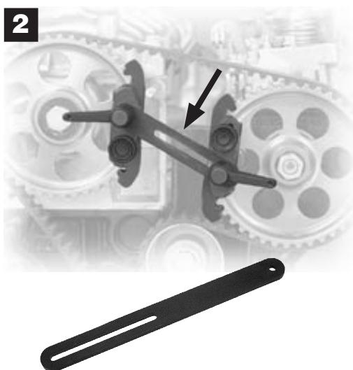
**GB****Engine Timing/Sprocket Locking Device**
