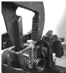
Using a suitable pair of adjustable pliers fit the jaws to span across from the back of tool to the front of the torsion spring plate.
