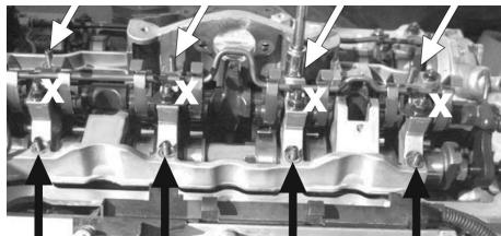
**CAREFULLY SELECT WHICH OF THE NUTS MUST BE RELEASED IN ORDER TO REMOVE THE CAMSHAFT/CARRIER BRACKET ASSEMBLY.**
