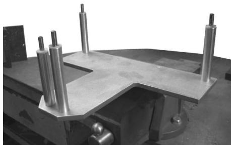
Assemble the Mounting Fixture and clamp it in a suitable vice on the workshop bench.
