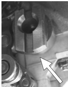
**IMPORTANT:** When installing the inlet camshaft, the curved edge of the rectangular section at the rear of the camshaft MUST BE pointing downwards in order that the camshaft is in the correct position when the carrier bracket is installed in the cylinder head.
