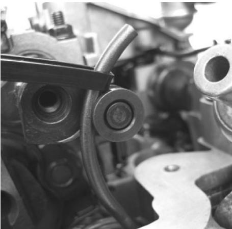
Rotate the eccentric shaft, via the hexagon, to reduce the amount of tension on the torsion spring. Fit a cable tie to the spring and pull back slightly to lift the spring off its roller and then allow the spring to move slowly forward and passed the roller, to relieve the tension.
