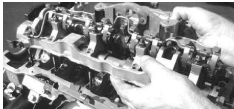
For further dismantling, the camshaft/cARRIER bracket must be carefully removed from the cylinder head
