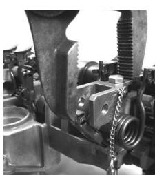
Carefully and slowly, in a controlled manner, allow the Plier jaws to open in order to release the torsion spring pressure fully.
