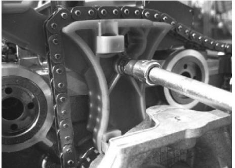
Unscrew and remove the upper screw of the chain guide.
