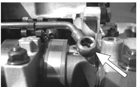
Detach the pulse generator plug for the inlet camshaft.
