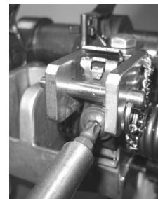
Maintain the spring in this position with the Pliers and Slide the Safety Pin in place - fully through both sides of the Tool. The Safety Pin will restrict the torsion spring's movement, backwards.
