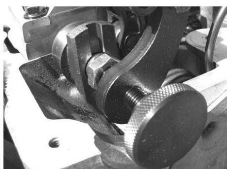
Fit D817 Camshaft Securing Tool (Rear) on to the back of the inlet camshaft by screwing its locking bolt into the internal thread in the end of the eccentric shaft (pinch tight only at first) and locating the 'domed' nut attached to the end of its locking screw, in to the large countersink of the hole in the rectangular section in the rear of the inlet camshaft. Tighten the 'domed nut' screw, by hand, to 'lock' the tool onto the camshaft. Tighten the locking bolt into the eccentric shaft.
