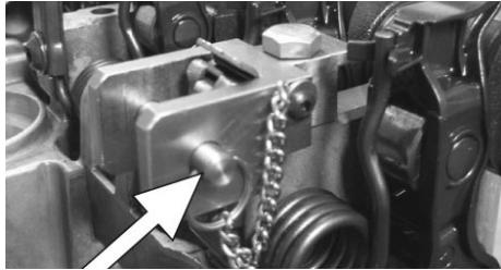
Slide the Safety Pin fully in to place - through both sides of the Tool, The Safety Pin will restrict the torsion spring's movement backwards under tension, when the spring retaining screw is removed.
