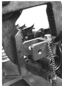
Carefully and slowly, in a controlled manner, close the Plier jaws to compress the spring to a position where the spring plate goes beyond the holes in the Tool which accept the Safety Pin.
