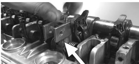
Fit D814 Tool to the carrier bracket and secure in place by inserting its bolt, from the top, through the Tool and through the Carrier Bracket. Fix with its nut from underneath - tighten nut.
