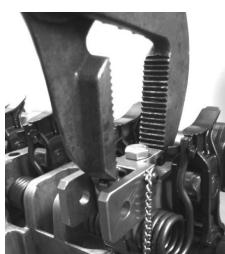
Carefully relieve the spring pressure off the Safety Pin by slightly closing the Plier jaws and whilst retaining the jaws in this position, pull out the Safety Pin.
