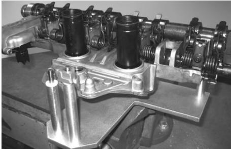
**IMPORTANT: INVERT the camshaft/cARRIER bracket assembly, so the inlet camshaft is uppermost.**
