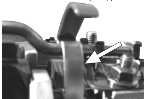
All 8 x Clamps of D818 Set **MUST BE** fitted. Attach the Clamps to the bottom of the levers and secure the top of the Clamps on to the oil supply pipe.
