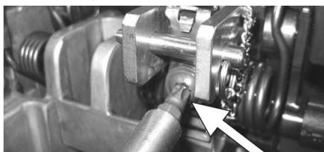
Slowly unscrew and remove the torsion spring retaining screw (Tx30) so that the spring plate pushes against the Safety Pin.
