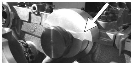
Fit D816 Camshaft Securing Tool (Front) onto the front of the inlet camshaft ensuring it **locates fully and correctly** onto 'lip' of the cylinder head and secure in place with its locking screw **fully** screwed in to the internal thread in the end of the camshaft.
