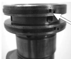
**Inlet camshaft** - Always check condition of the Plain Compression rings, they can break easily. To install - carefully pull apart and fit from the front. Press ring from one side to engage the catch on the other side.
