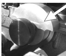
Fit Securing Tools D816 and D817 to fix each end of the inlet camshaft to the carrier bracket. Lubricate Intermediate Levers with engine oil and install
