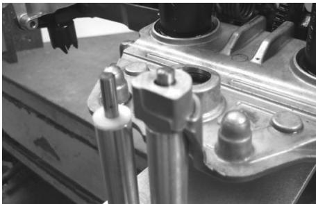
Locate the carrier bracket assembly on to the top of the pillars of D819 Mounting Fixture.
